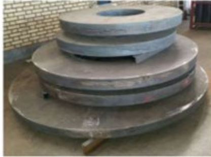
7- These multiring diaphragms are novel. In addition, these diaphragms are made of metal sheets with different thicknesses and no casting needed that reduce the manufacturing costs and time.
