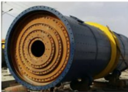
7- These multiring diaphragms are novel. In addition, these diaphragms are made of metal sheets with different thicknesses and no casting needed that reduce the manufacturing costs and time.
