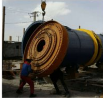
7- These multiring diaphragms are novel. In addition, these diaphragms are made of metal sheets with different thicknesses and no casting needed that reduce the manufacturing costs and time.
